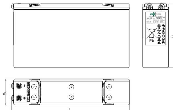
Tightening torque of terminal screw: 15 Nm - 133 lbf in
