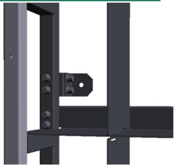
> To adjust the wall distance precisely to the surroundings, the L-bracket 2 is screwed in place using M8 x 20 spanner bolts and
