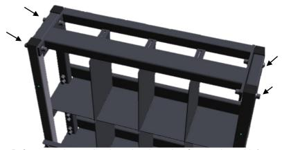
➤ Before you insert the batteries into the frame, the grid | Xtremetack seismic must be attached to the wall. To do this, the L-bracket 1 must be screwed in place using the M8 x 60 spanner bolts and the corresponding washers and nuts.
