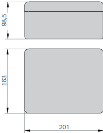
Figure 30: Dimensions of pump- and control unit
