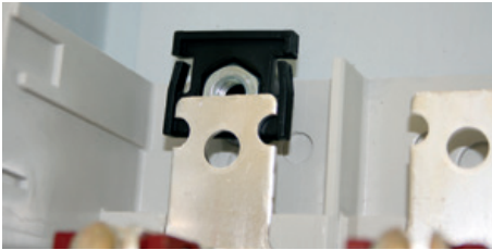
Figure 10: Fixing the nuts
