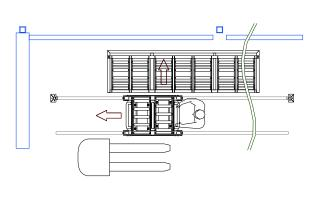
Once the track is secured in place and the height adjustable transfer unit with pallet truck is positioned on the track the end stops must be installed to both ends of the Convex D track, drill through the holes using an M10 SDS drill bit and fasten them down using the M10 x 75 Through bolts supplied.
