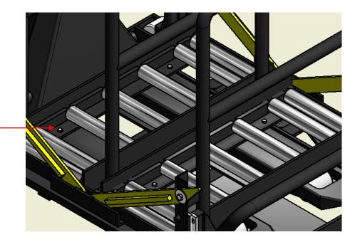
4 Off Bolts To Remove Roller Carriage
