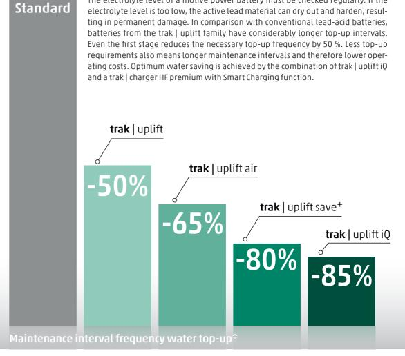
The electrolyte level of a motive power battery must be checked regularly. If the
